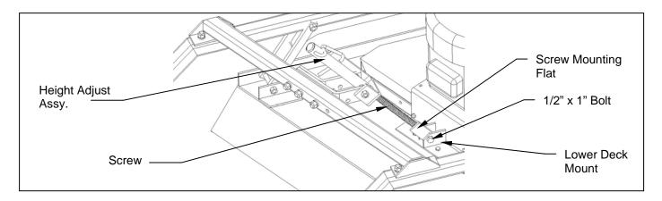
Figure 4: Height Adjust Assy. Installation
